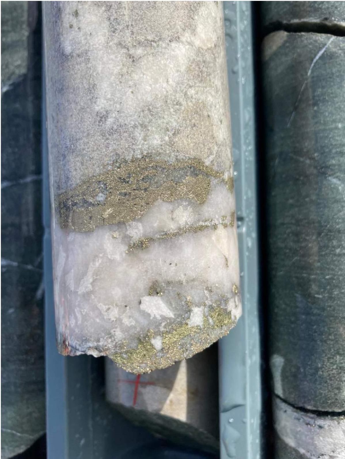
Photo 5: WRSDD0003, Chalcopyrite and pyrrhotite in quartz vein ~350 metres down hole.
