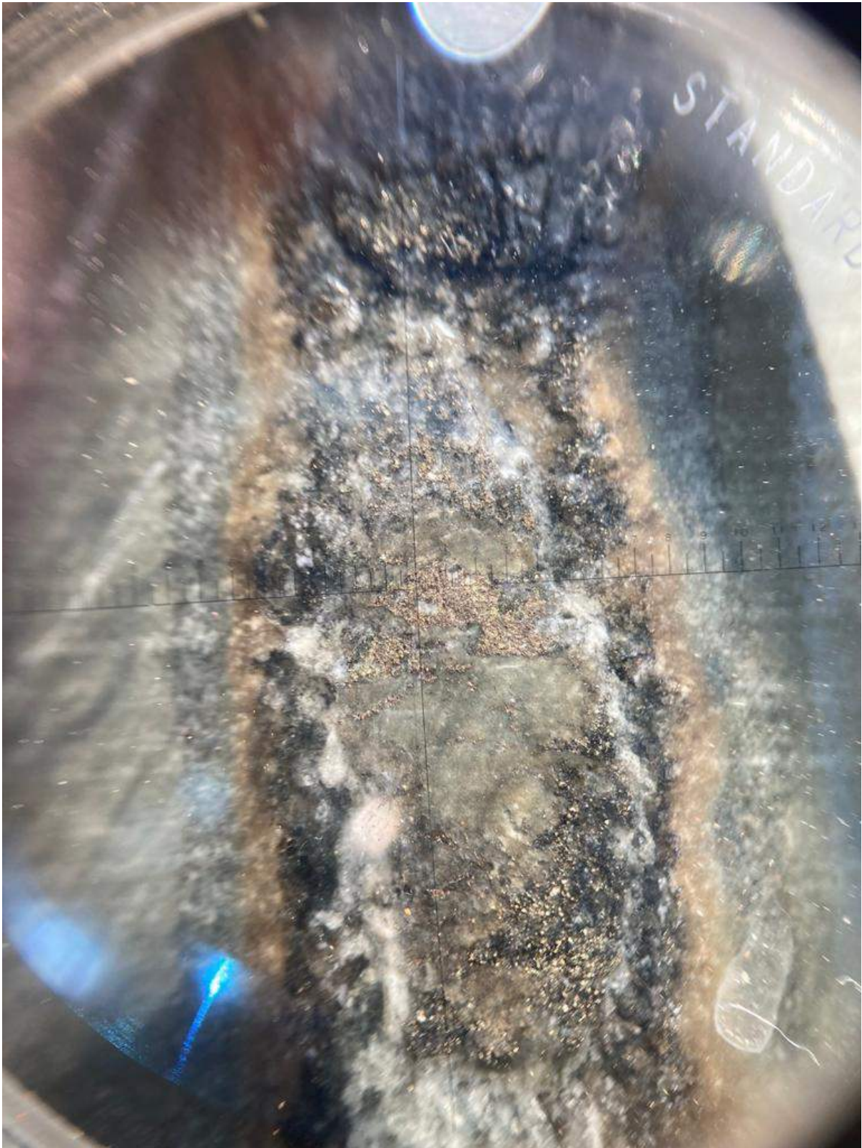
Photo 2: WRSDD0003, Pyrrhotite associated with albite - carbonate and biotite alteration at~ 345 metres
