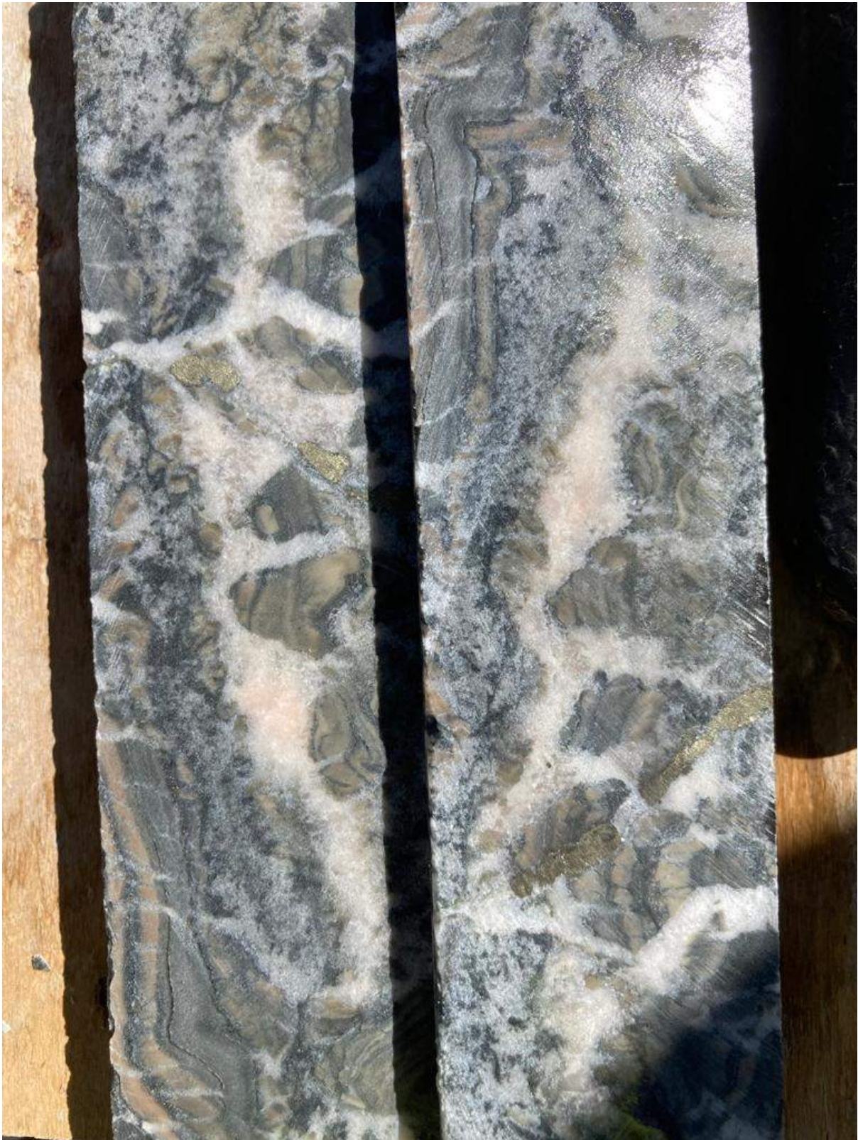
Photo 3: WRSDD0003, Brecciation around 280 - 290m. Note local clots of pyrite
