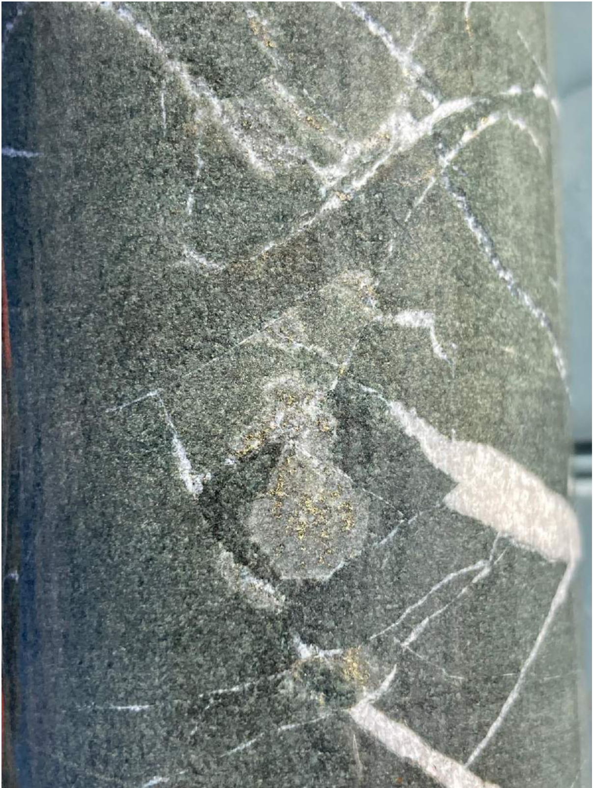
Photo 4: WRSDD0003, Chalcopyrite and pyrrhotite in quartz carbonate fractures and brecciation at ~345 metres
