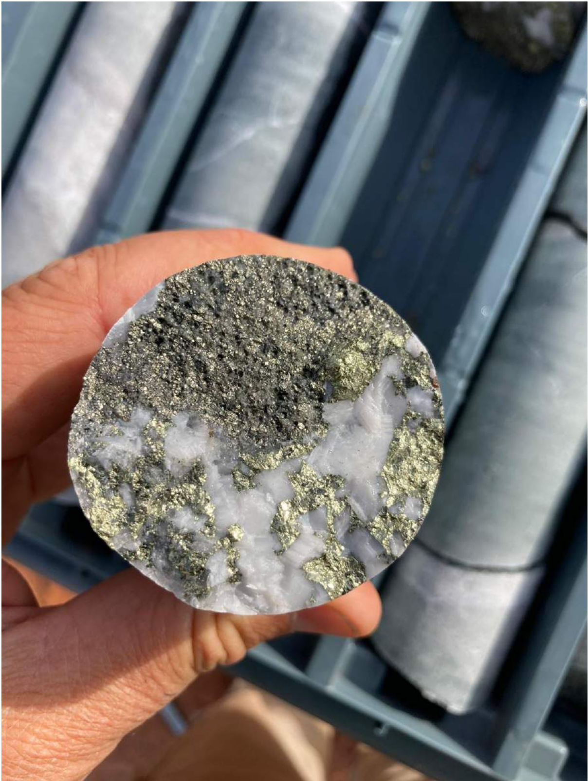
Photo 1: WRSDD0003, Chalcopyrite and pyrrhotite in quartz vein ~350m down hole.
