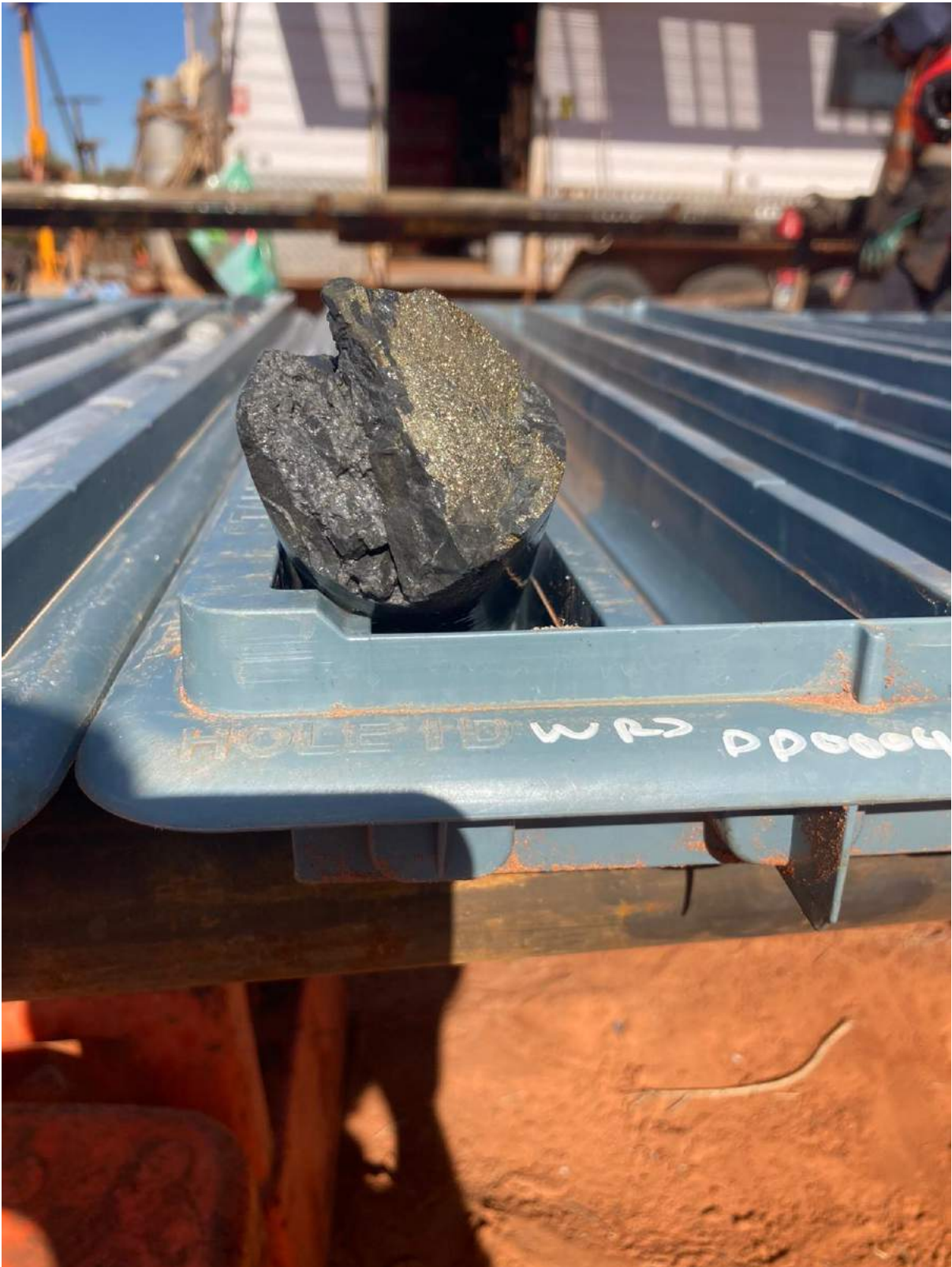
Photo 1: WRSDD0004, Chalcopyrite and pyrrhotite on joint surface at 57 metres.
