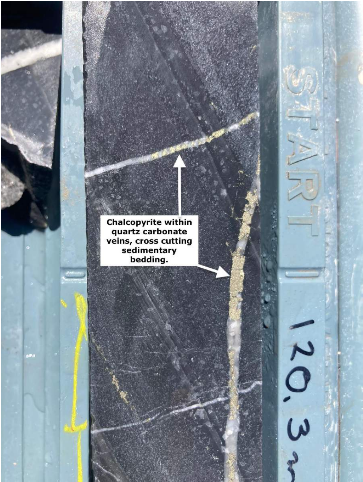
Photo 2: WRSDD0004, Chalcopyrite in veinlets cross cutting sedimentary bedding at 120.3 metres.
