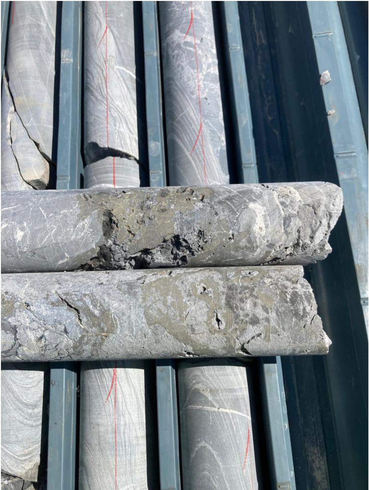
Photo 4: WRSDD0004, Chalcopyrite and pyrrhotite within a breccia and fault zone at 182-183 metres down hole.
