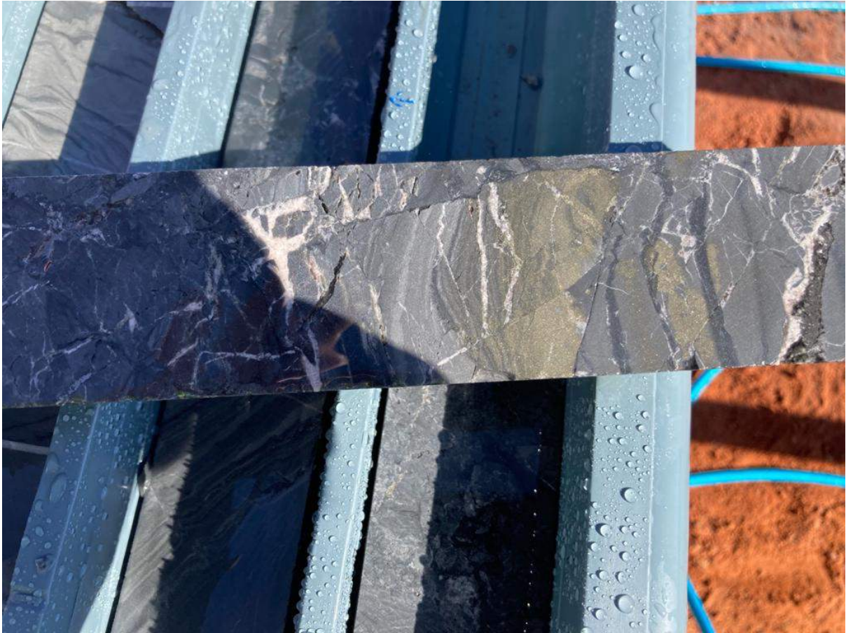
Photo 5: WRSDD0004, Cut core of photo 3 chalcopryrite and pyrrhotite within a breccia and fault zone at 182-183 metres down hole.
