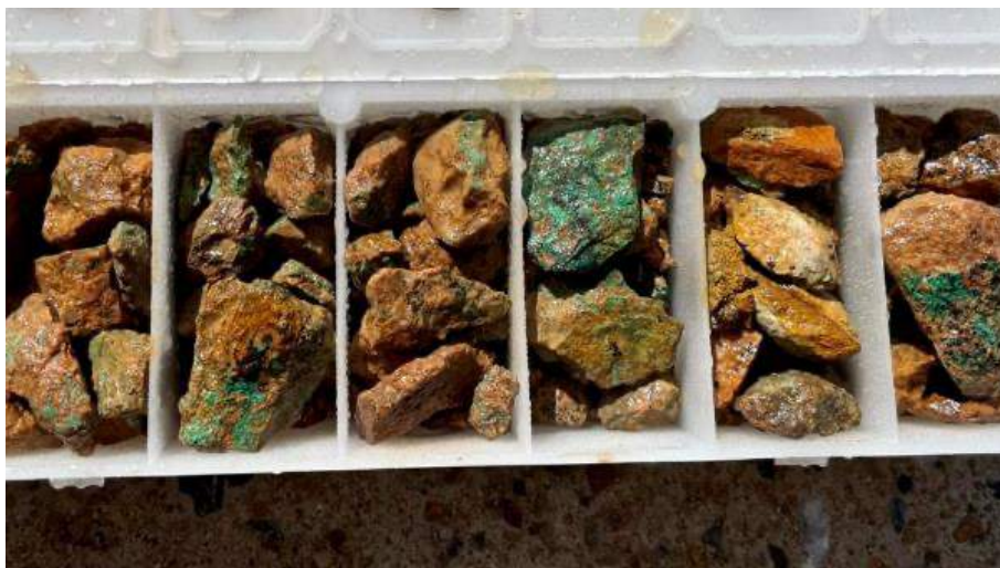
Figure 4: Reverse circulation percussion chips from Halo SE, Hole # 21, copper oxide zone containing abundant malachite (from 0m-19m).
