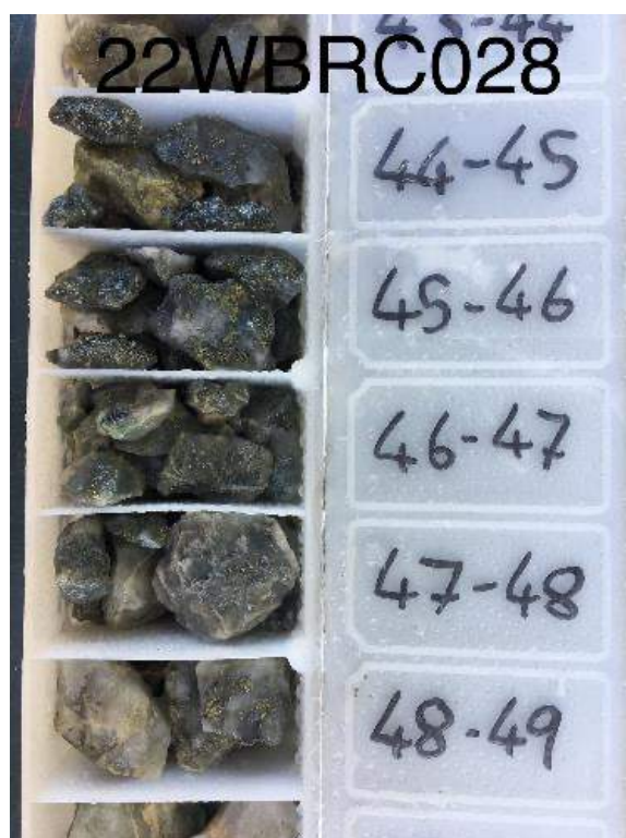
Figure 7: Reverse circulation percussion chips (44m-49m) from Grassy Oaky
