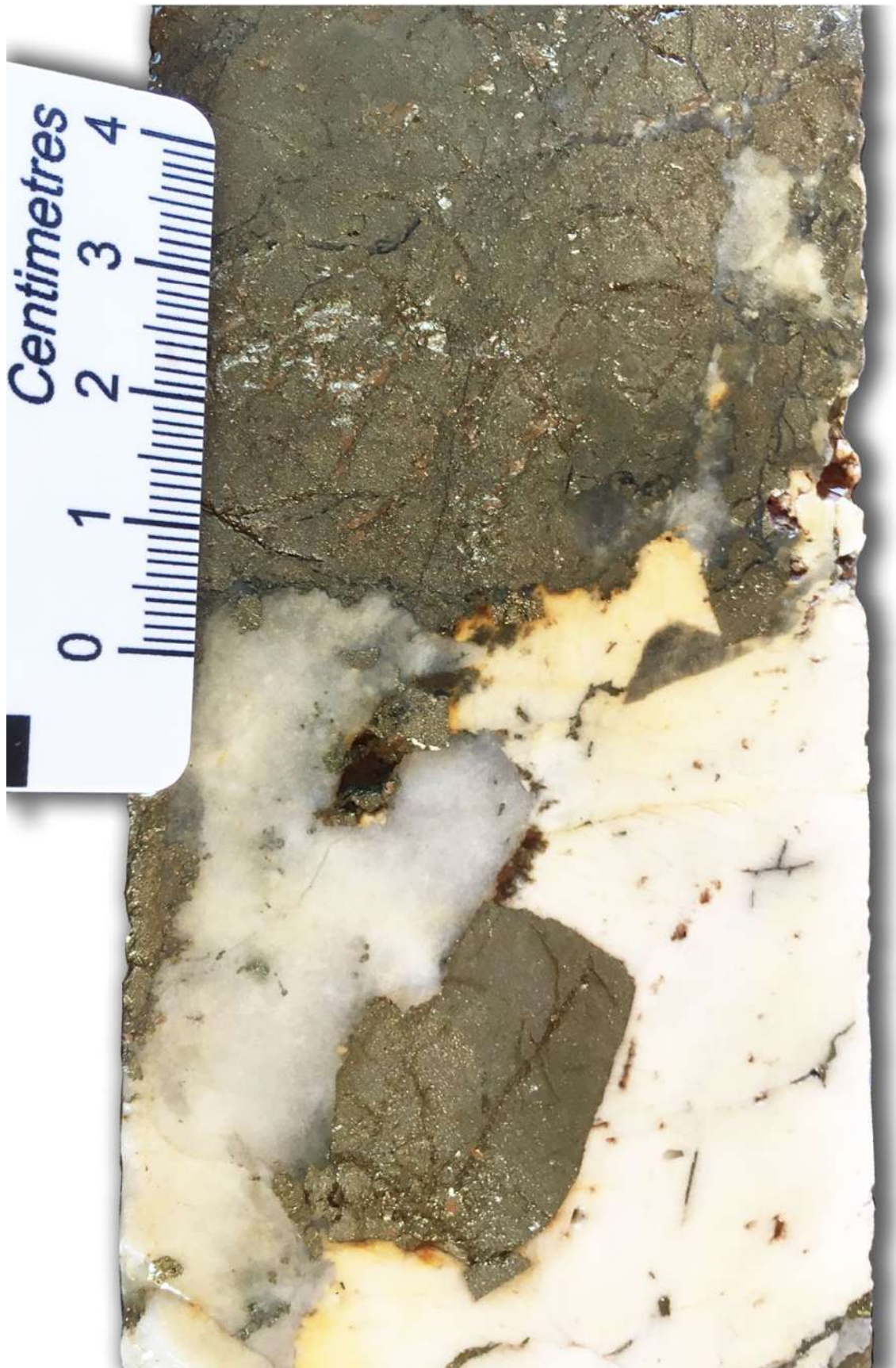
Figure 7: Example of Quartz-carbonate sulphide reef in drill core at Telfer (Source: Mike Porter 2019, Website: http://portergeo.com.au/database/mineinfo.asp?mineid=mn224 )
