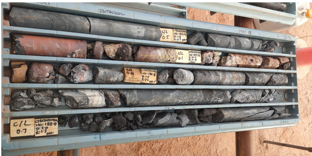
Figure 2 – Drill tray containing oxidised, brecciated gossanous zone from 184-189m
