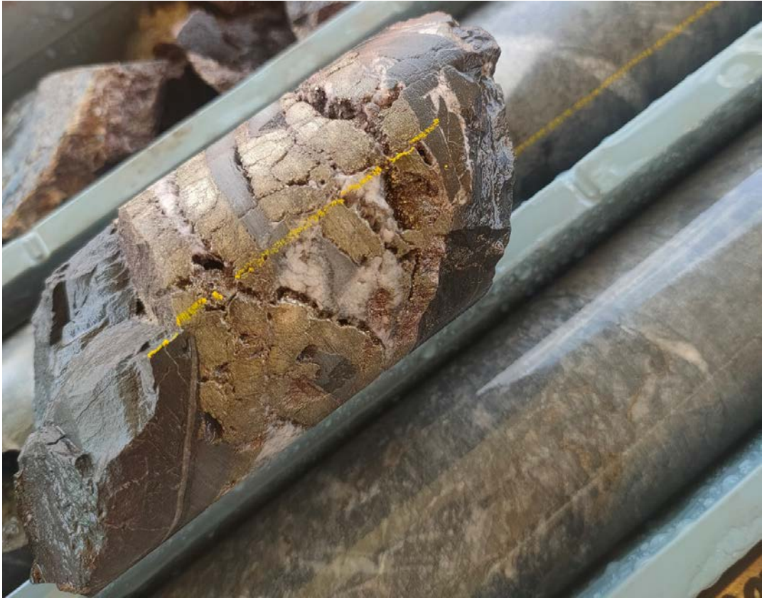
Figure 3 – core containing quartz carbonate vein, pyrite and minor chalcopyrite 134.2m
