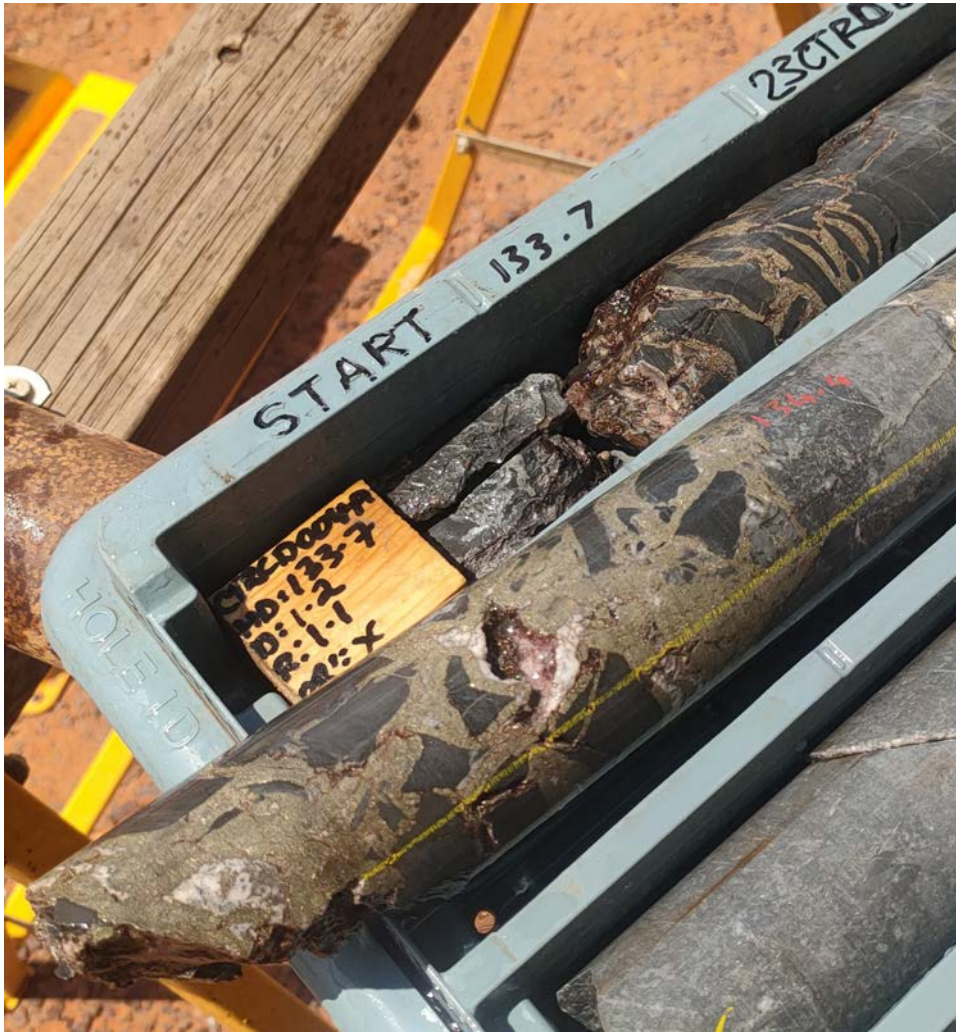
Figure 1 – Brecciated shale with substantial pyrite (+ minor chalcopyrite) matrix 133.7m
