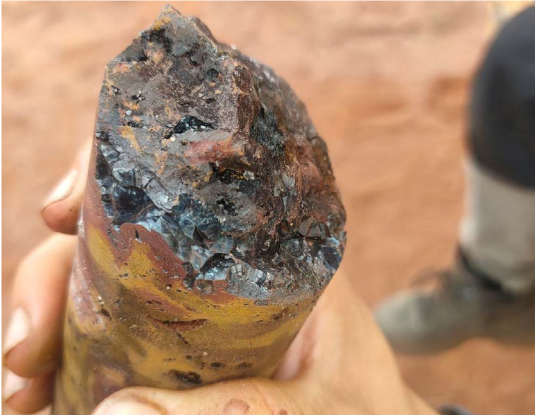
Figure 4 – Oxidised brecciated core with Goethite, Haematite and Manganese Oxides 186m.
