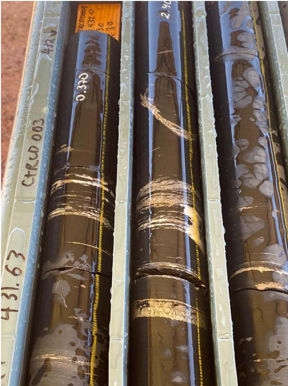
Photo 3 – Lamination parallel Pyrite & pyrrhotite with carbonate veining
