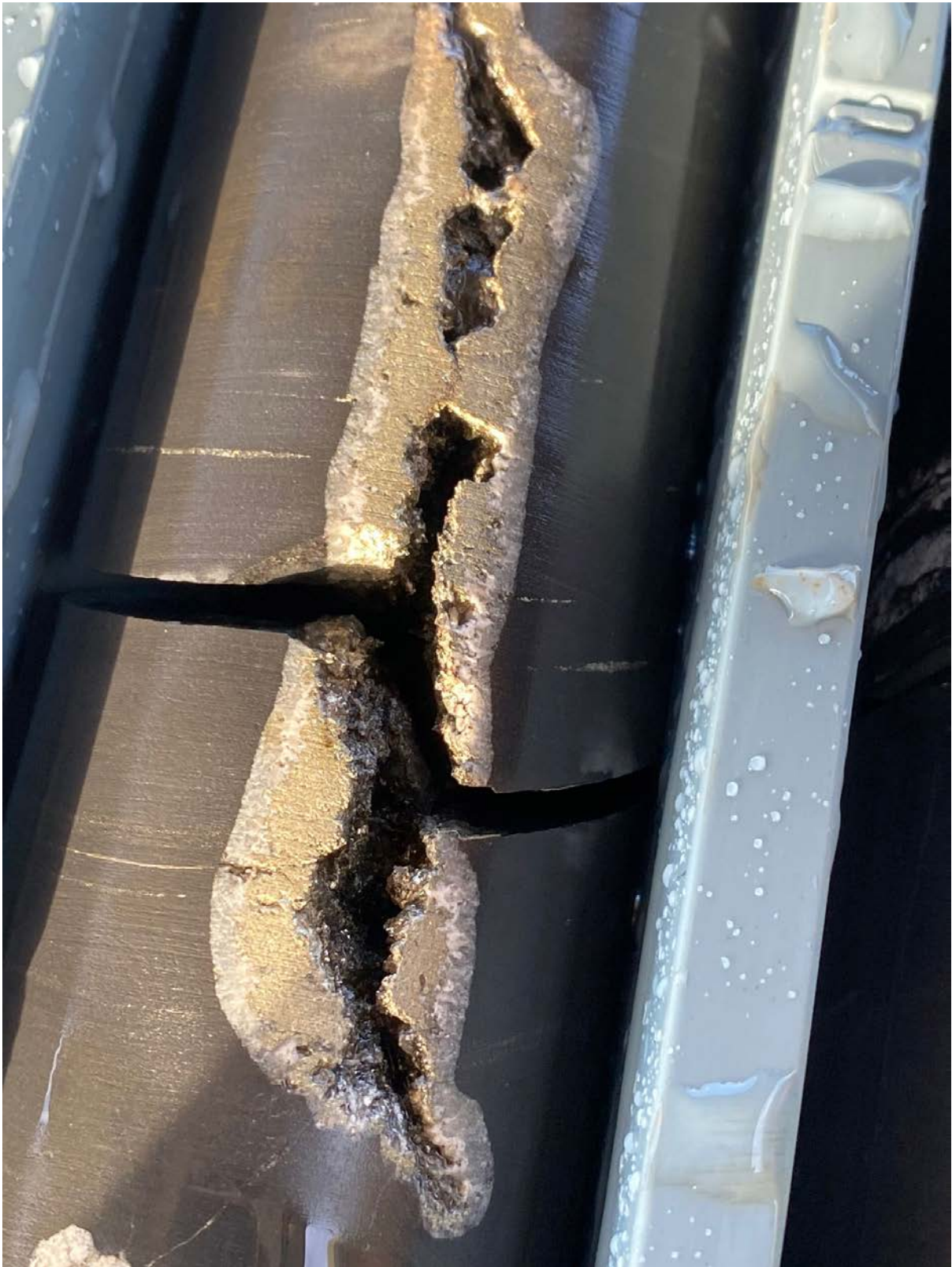
Photo 6 –Pyrite dissemination with cavities within a thicker zone of qtz-carb-silicious veining 368-370m
