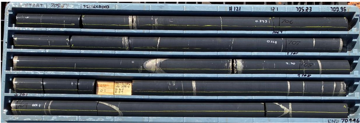
Photo 2 - Pyrite & Pyrrhotite +/- minor sphalerite banded and veined black shale interval
