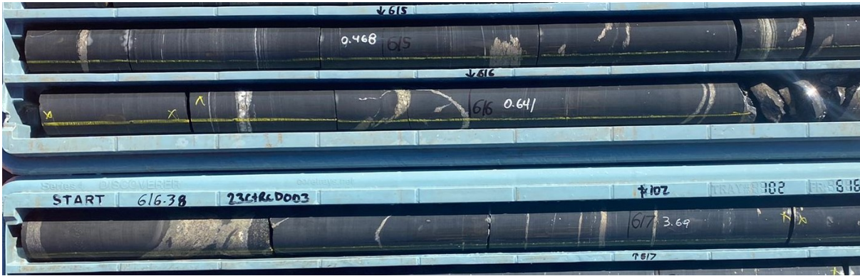
Photo 1 - Pyrite & Pyrrhotite banded and veined shale interval with initial scans from XRF reading elevated base metals
