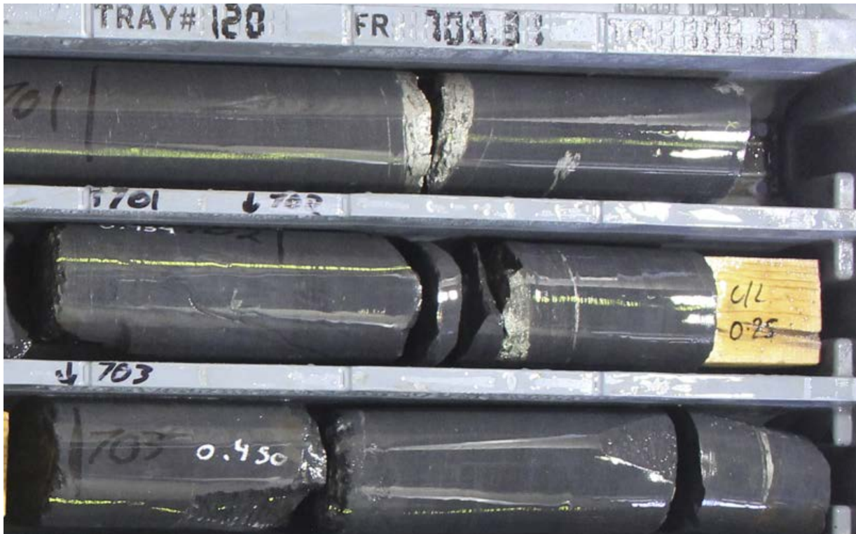
Picture 1 - 23CTRCD003 – Black shale hosting Pyrite-pyrrhotite veinlets
