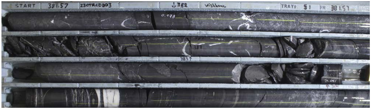
Picture 3 - 23CTRCD003 – Black shale, semi brecciated with carbonate-quartz veining hosting up to 1.3g/t Ag
