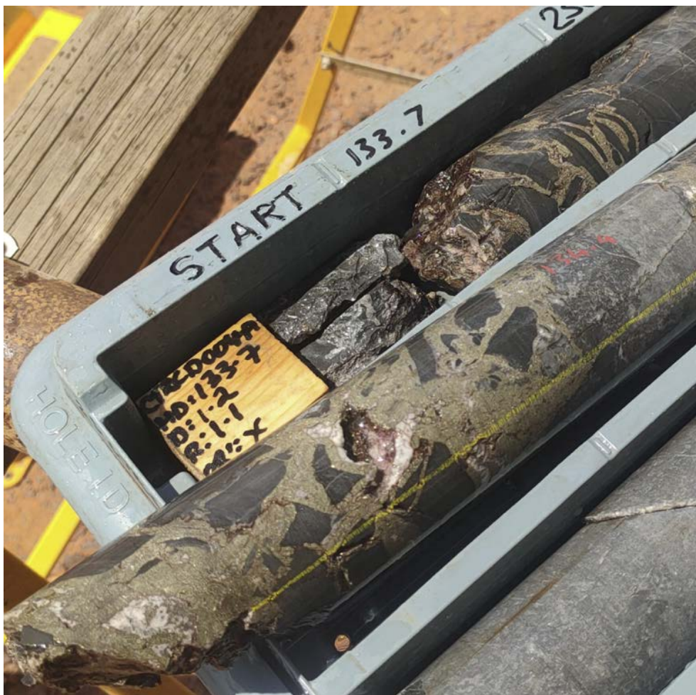
Picture 5 - 23CTRCD004A – Breccia infill pyrite, trace chalcopyrite containing up to 1.2g/t Ag
