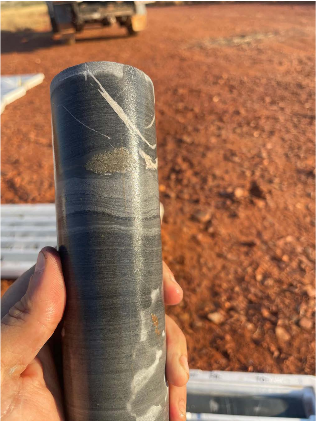
Figure 6: Quartz carbonate veining including chalcopyrite and pyrite sulphides at 754.2m
