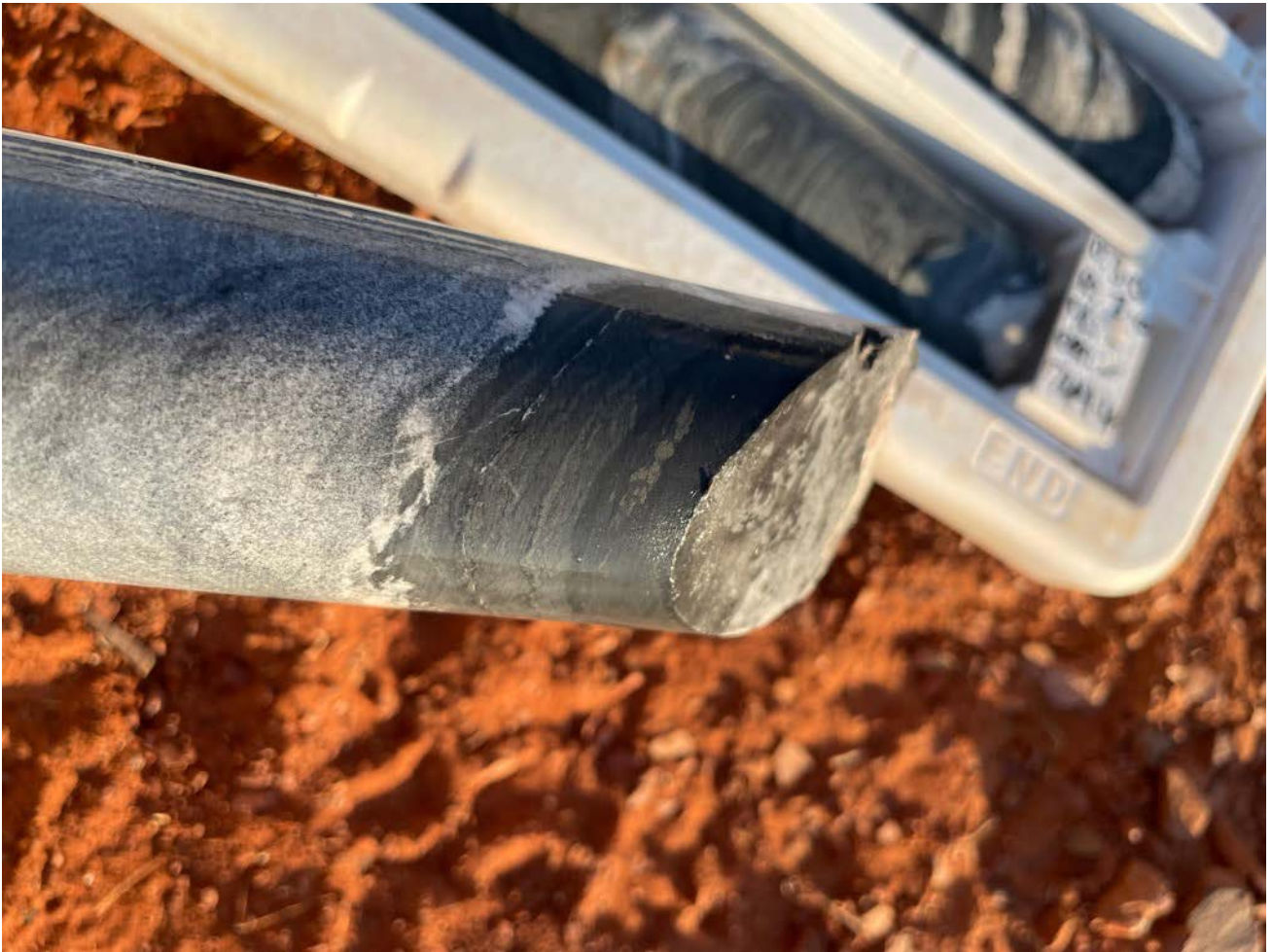
Figure 9: Quartz carbonate veining including chalcopyrite and pyrite sulphides at 740m.
