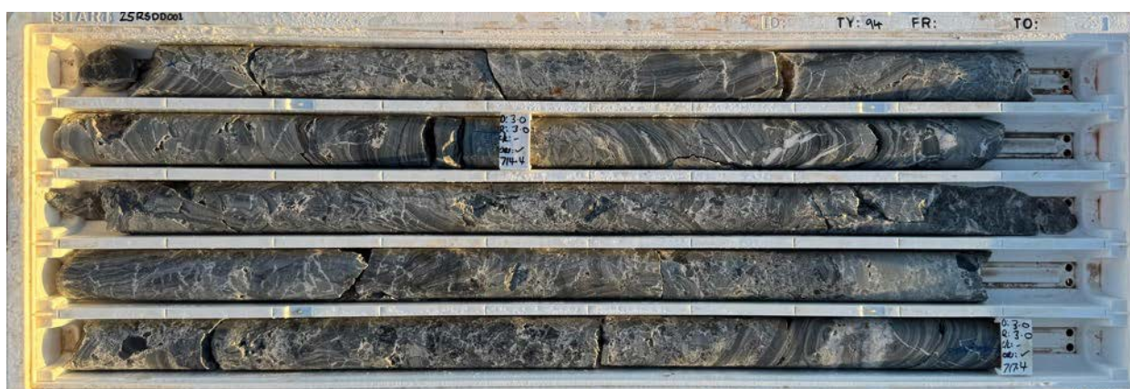
Figure 2: Breccia with chalcopyrite and pyrite sulphides, Core from 713-717m.
