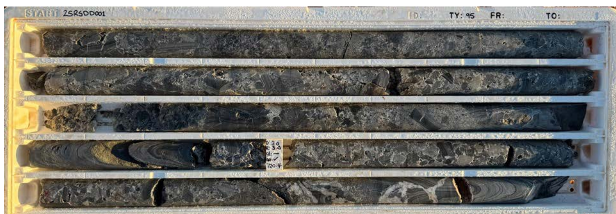
Figure 3: Breccia with chalcopyrite and pyrite sulphides, Core from 717-722m.
