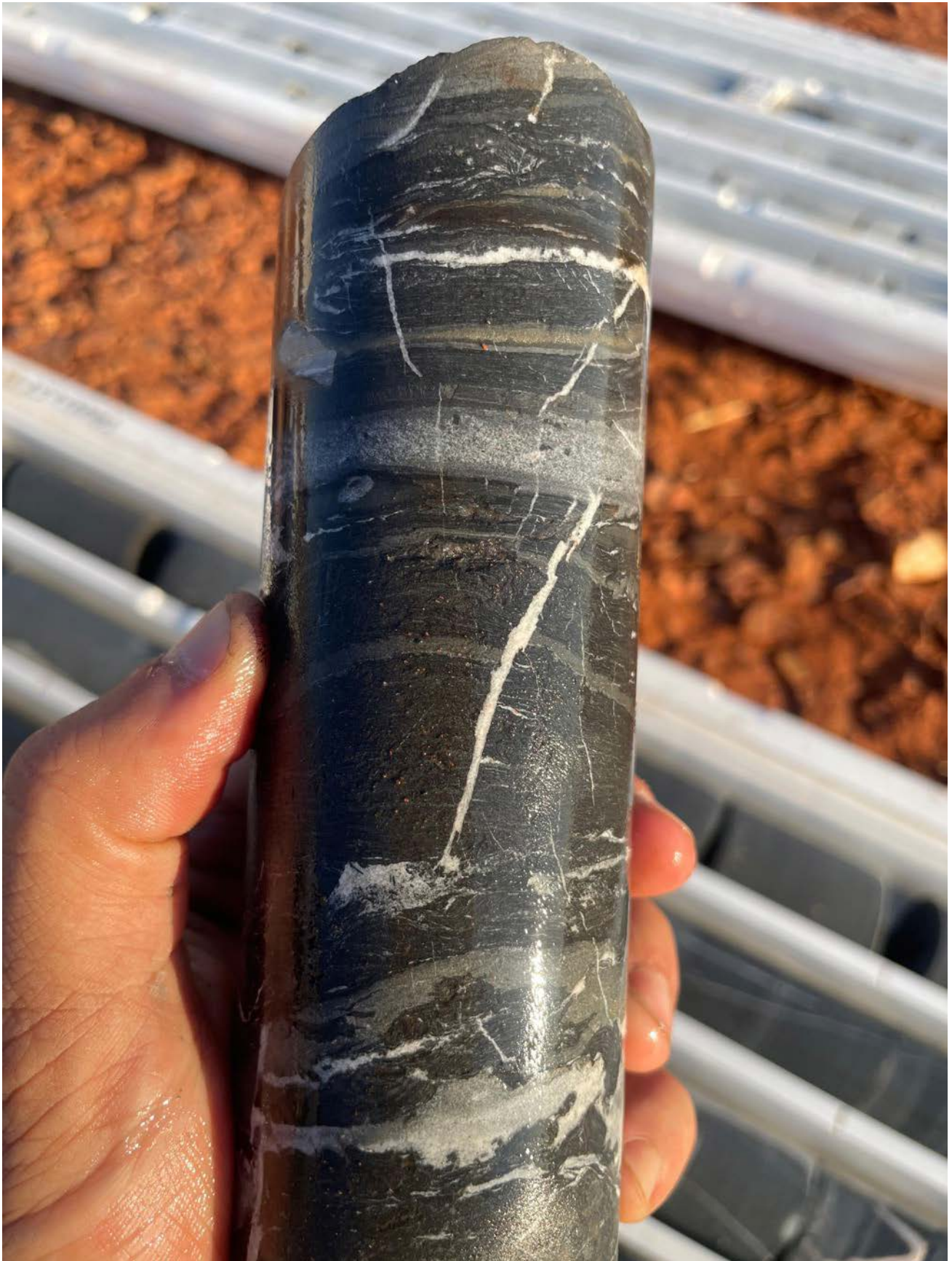
Figure 5: Quartz carbonate veining including chalcopyrite and pyrite sulphides at 756.5m
