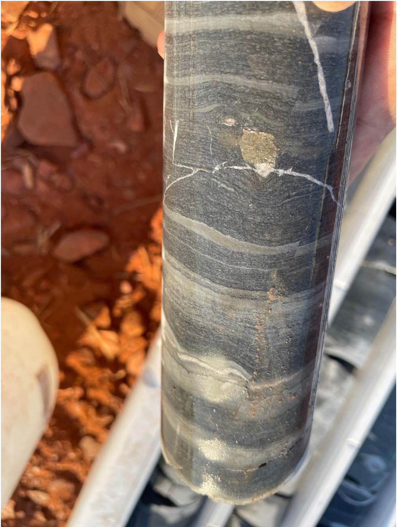
Figure 8: Quartz carbonate veining including chalcopyrite and pyrite sulphides at 751m.
