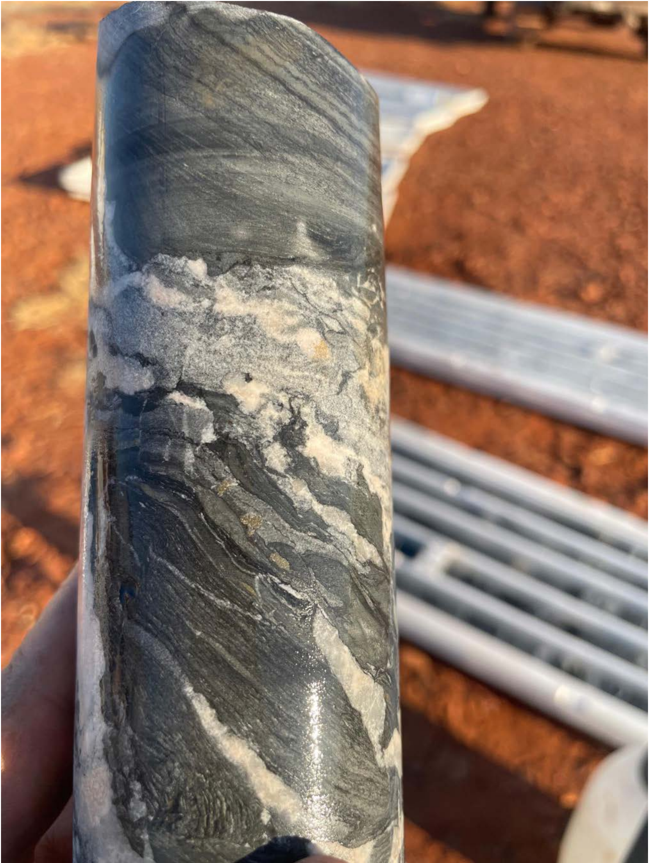
Figure 4: Quartz carbonate veining including chalcopyrite and pyrite sulphides at 746.2m.
