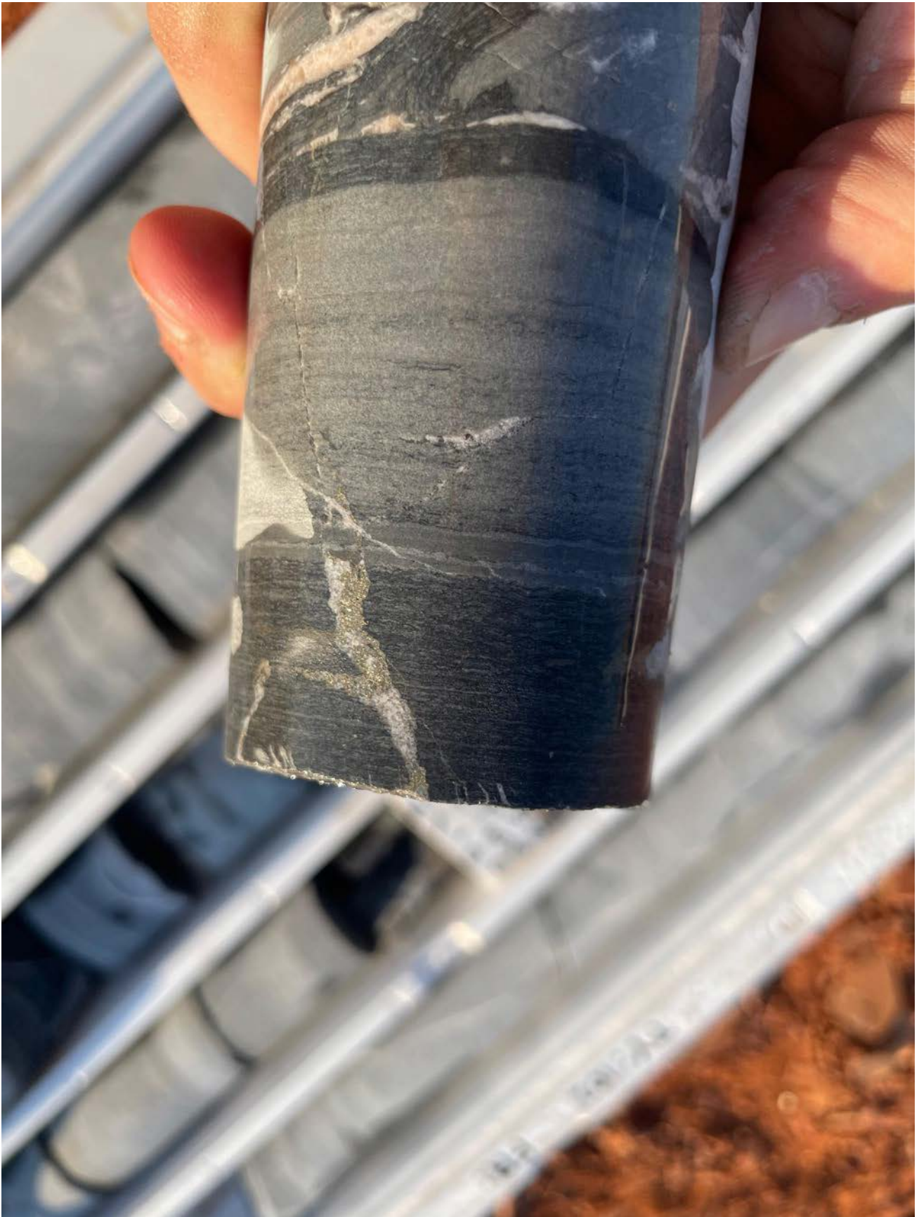
Figure 7: Quartz carbonate veining including chalcopyrite and pyrite sulphides at 751.4m
