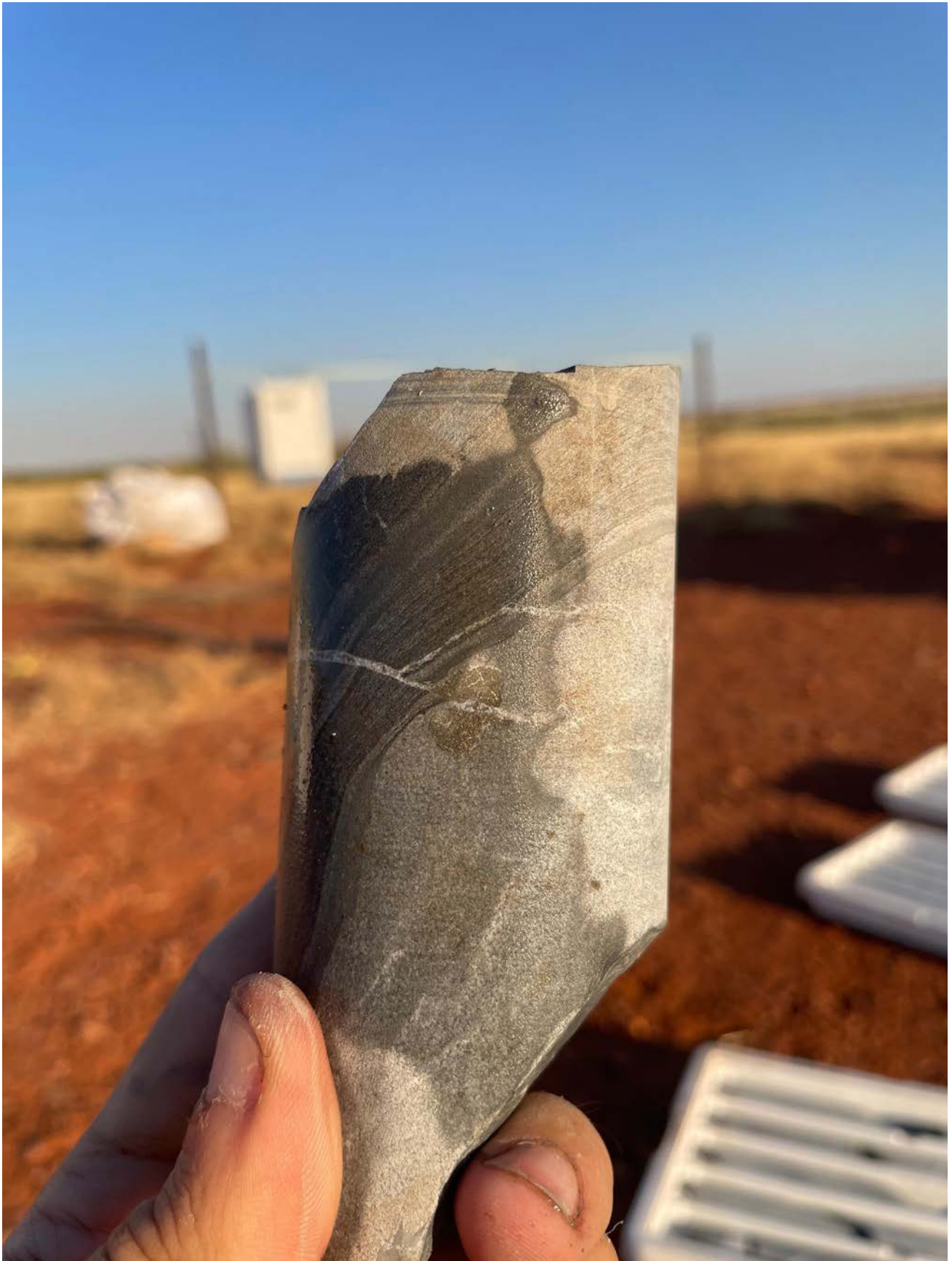
Figure 10: Quartz carbonate veining including chalcopyrite and pyrite sulphides at 738.4m
