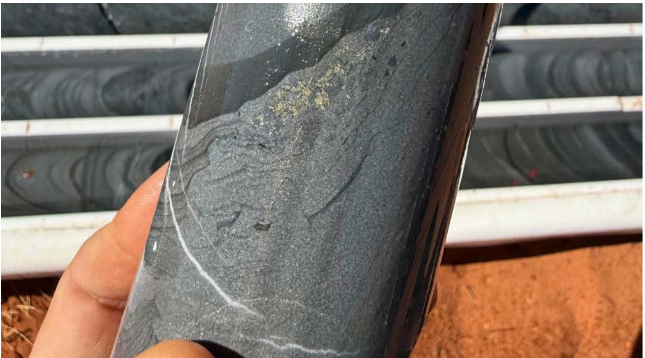
Figure 5: Pyrite with chalcopyrite in sandstone. (Core at 561.5m)
