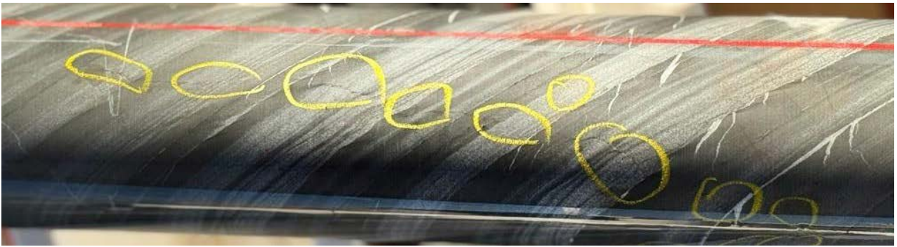
Figure 3: Fractures in siltstone and sandstone are filled with pyrite and trace chalcopyrite. (Core at 552.20m)
