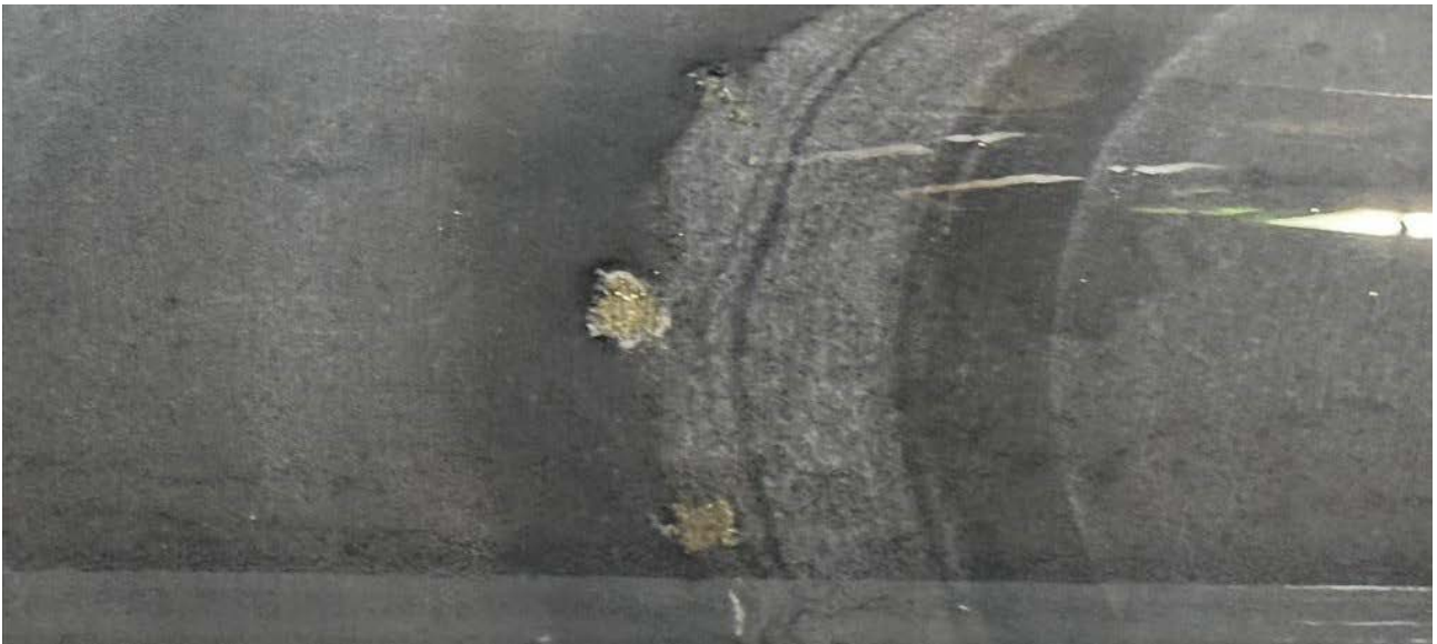
Figure 6: Metamorphism of the siltstone and sandstone creating more glassy and bleached appearance, with pyrite sulphide. (Core from 571.7m)
