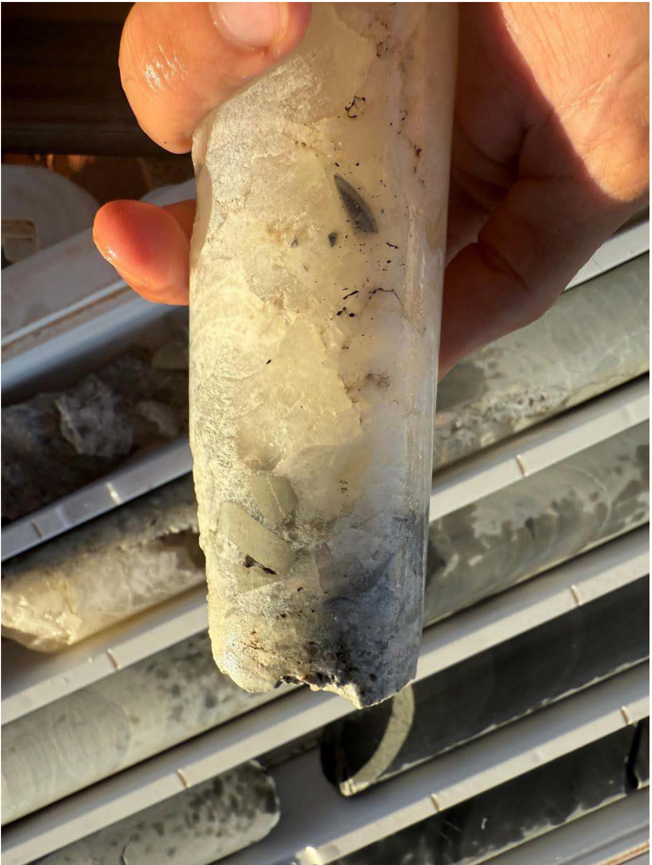
Figure 11: Massive coarse grained carbonate vein with minor quartz concentrated on the edges of the vein. There is fine grained disseminated pyrite on the surfaces of vugs within the vein. (Core at 579.6m)
