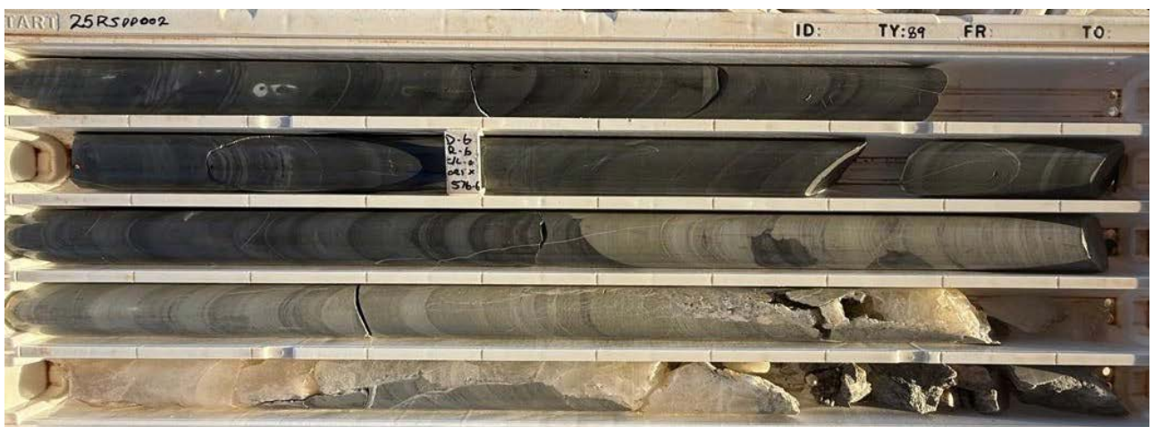
Figure 8: Metamorphism and bleaching of sediments from 577.6m, then from 578.8 massive coarse grained carbonate vein with minor quartz concentrated on the edges of the vein. There is fine grained disseminated pyrite on the surfaces of vugs within the vein. (Core from 575-580m)
