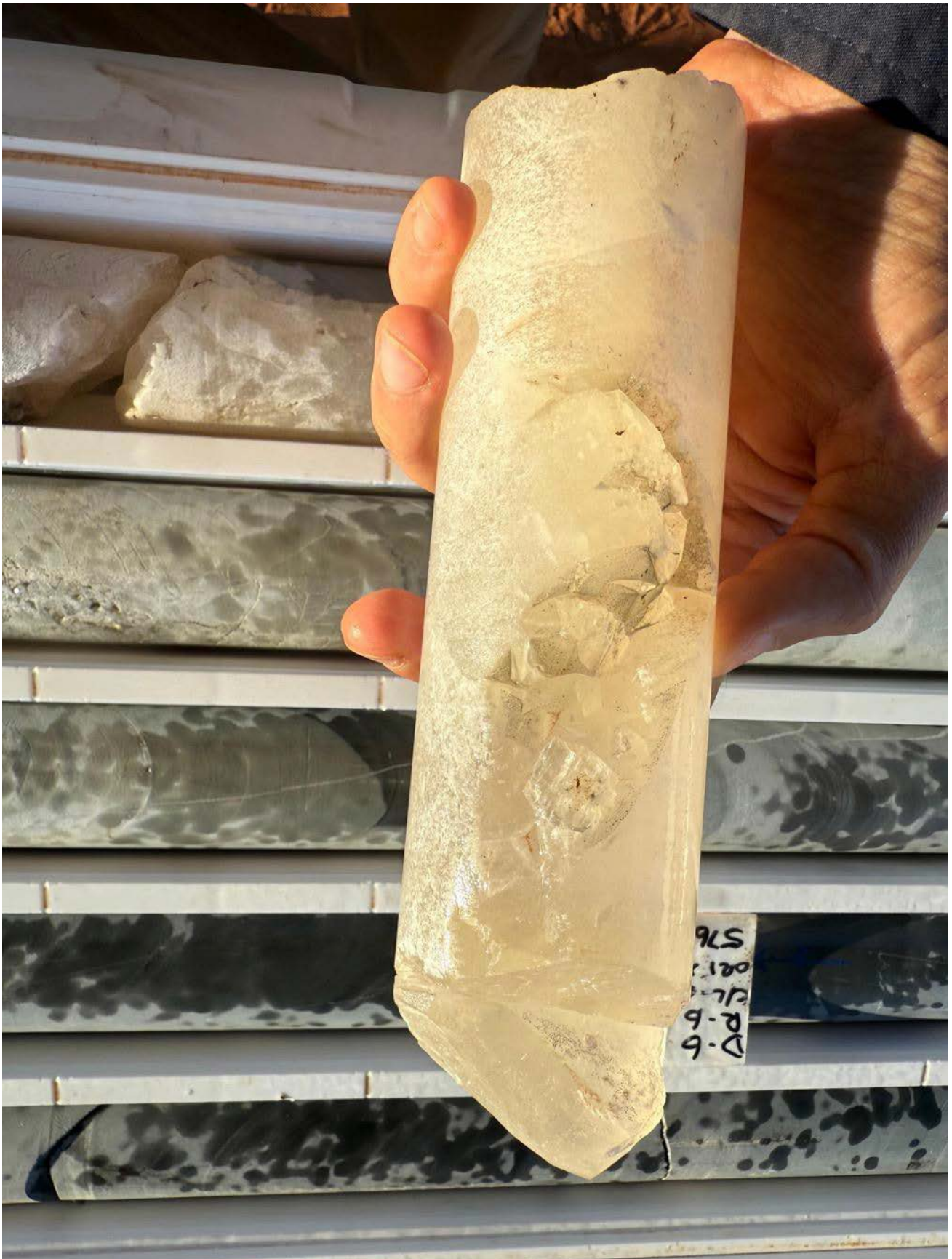
Figure 10: Massive coarse grained carbonate vein with minor quartz concentrated on the edges of the vein. There is fine grained disseminated pyrite on the surfaces of vugs within the vein. (Core at 579m)
