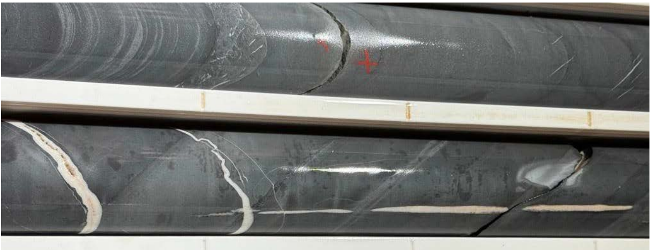
Figure 7: Metamorphism of the siltstone and sandstone creating more glassy and bleached appearance, with carbonate vugs cross cutting bedding. (Core from 573m)
