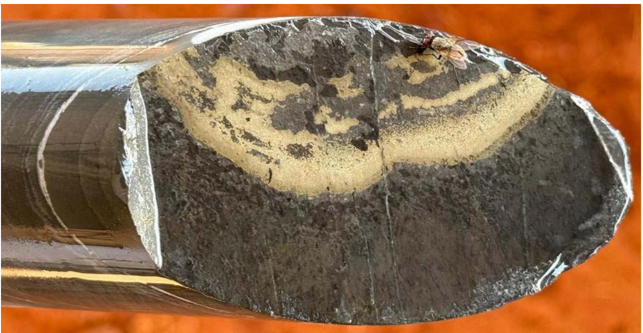
Figure 2: Fracture in siltstone filled with pyrite, with fly for scale. (Core at 548.50m)
