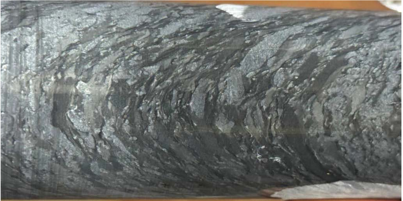
Figure 4: Breccia texture within deformed siltstone containing pyrite. (Core from 559.17m - 560.53m)
