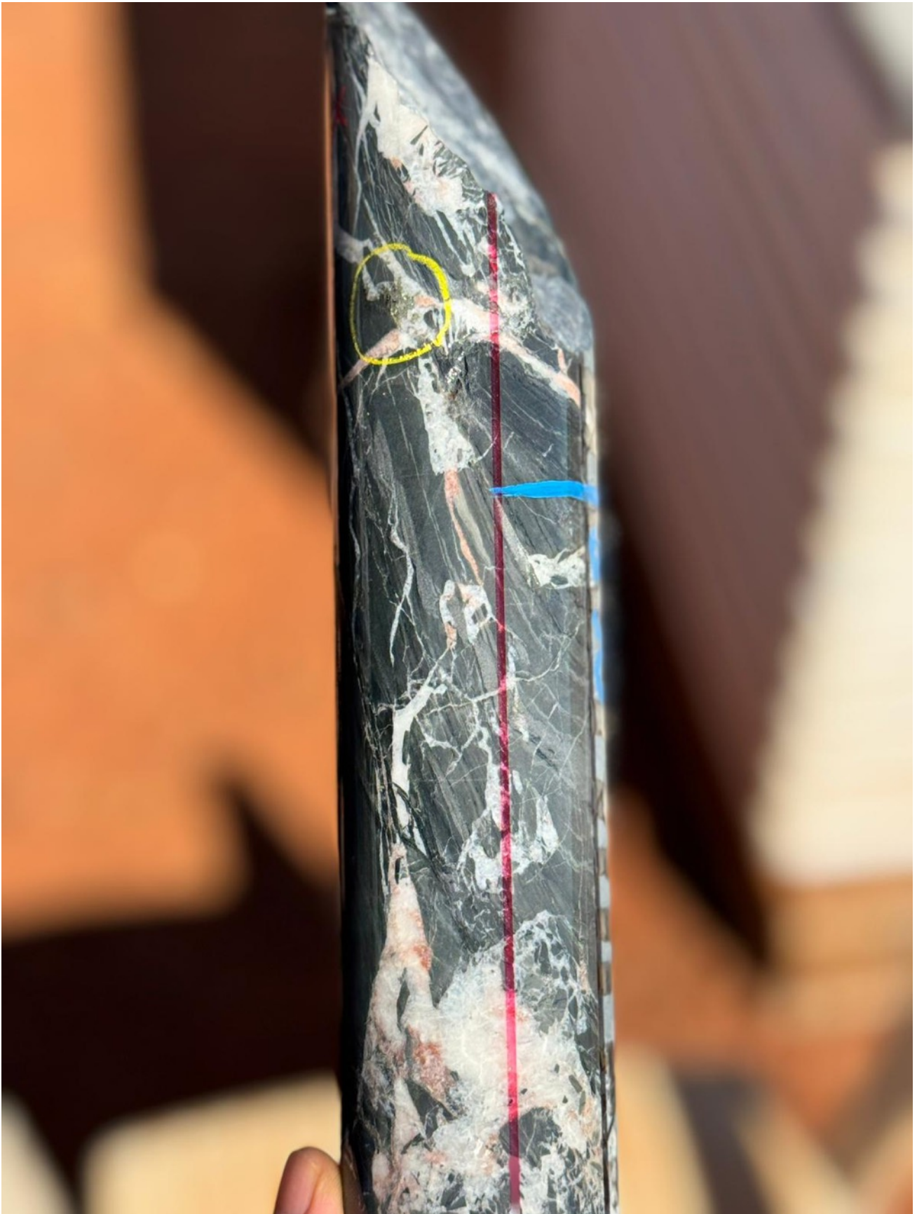
Figure 3: Fracturing of sediments with pyrite at 856m
