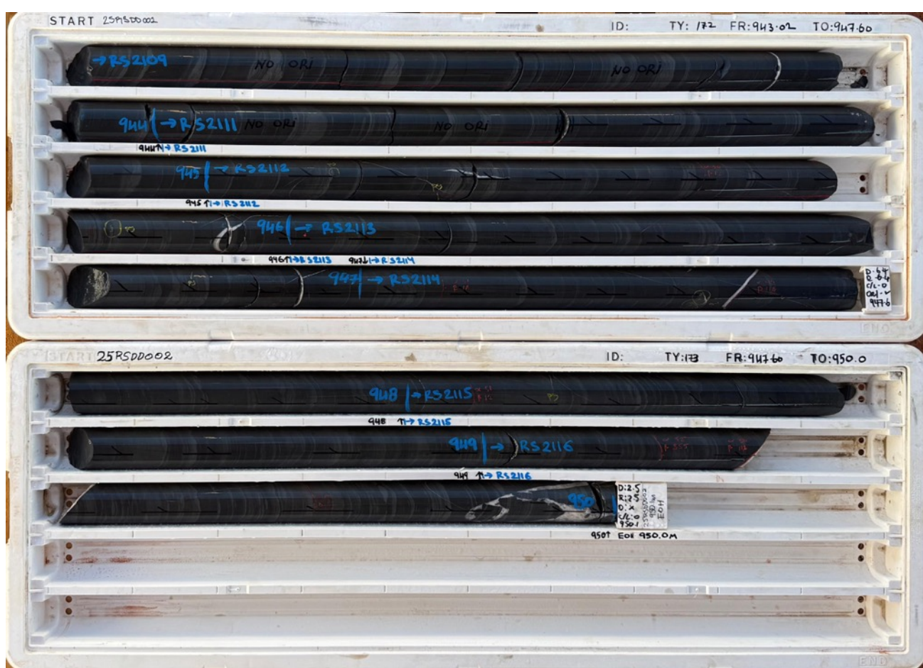
Figure 5: Minor fracturing of sediments with pyrite at 943m to 950m EOH.
