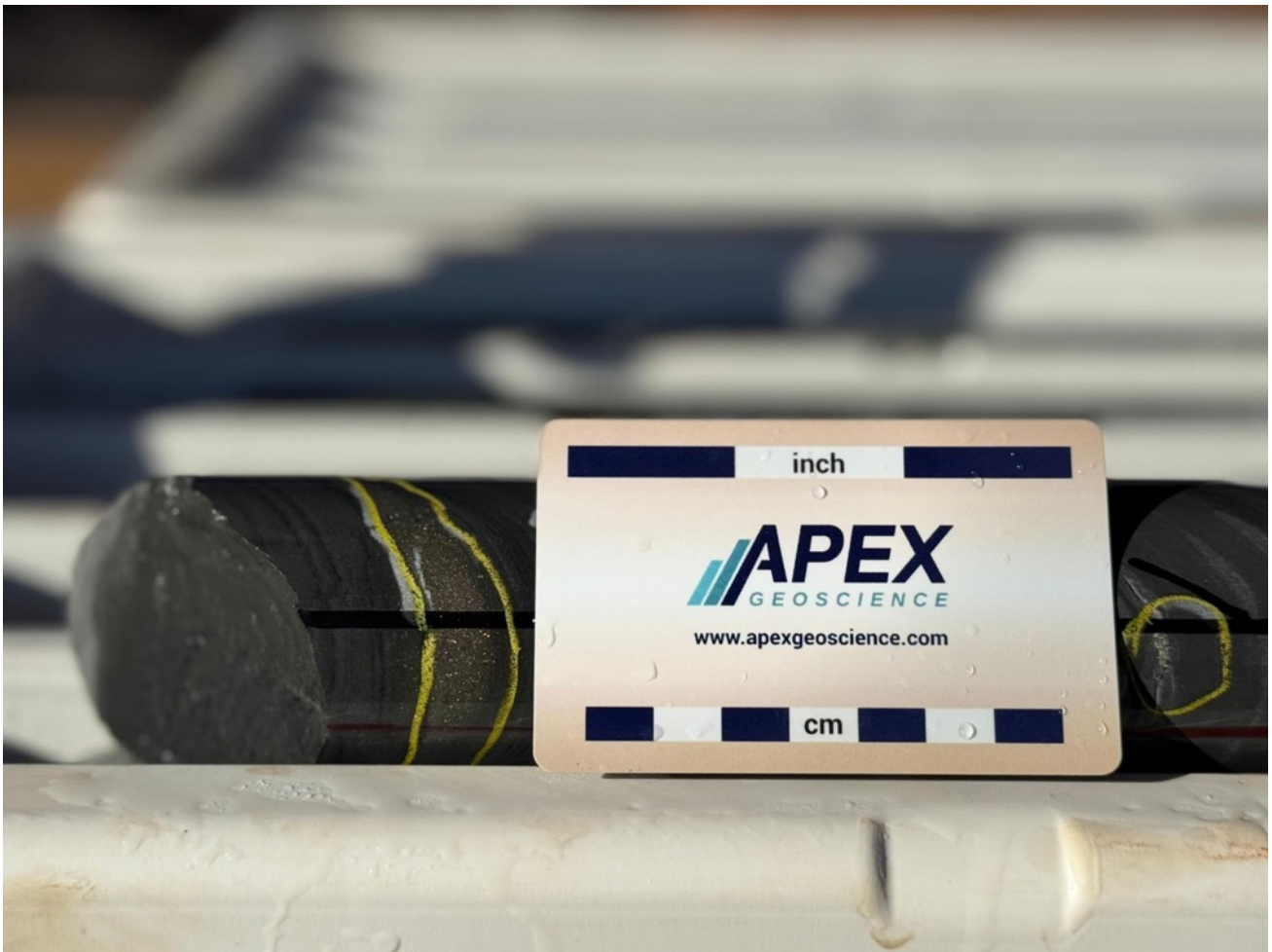
Figure 1: Pyrite vein at 850.75m
